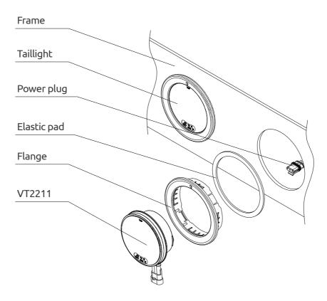
Step2: Connect the power cable, and install VT2211 into the tail light position.
