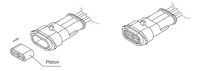
Step 4. Pull out the piston and house together from socket
