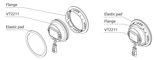
Step2: Connect the power cable, and install VT2211 into the tail light position.
